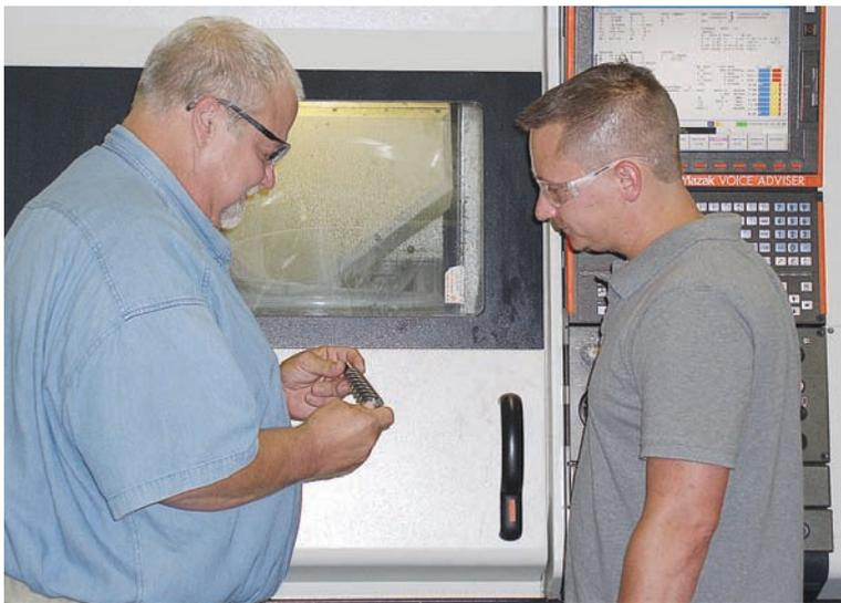
**Mike Mullins, abrasive-plated tool production supervisor (left) and operator Fred Wooley inspect one of Sunnen's HPH tools automatically programmed using the GibbsCAM plug-in for machining on the Mazak Integrex 100.**
