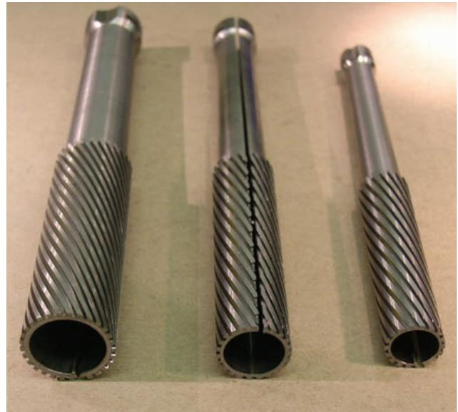
**Parts from the Sunnen CGT Krossgrinding) honing tool family show the variation in size and number of machined grooves. The GibbsCAM plug-in made programming easier and automatic, and cut programming time per part by 1.25 hr.**
